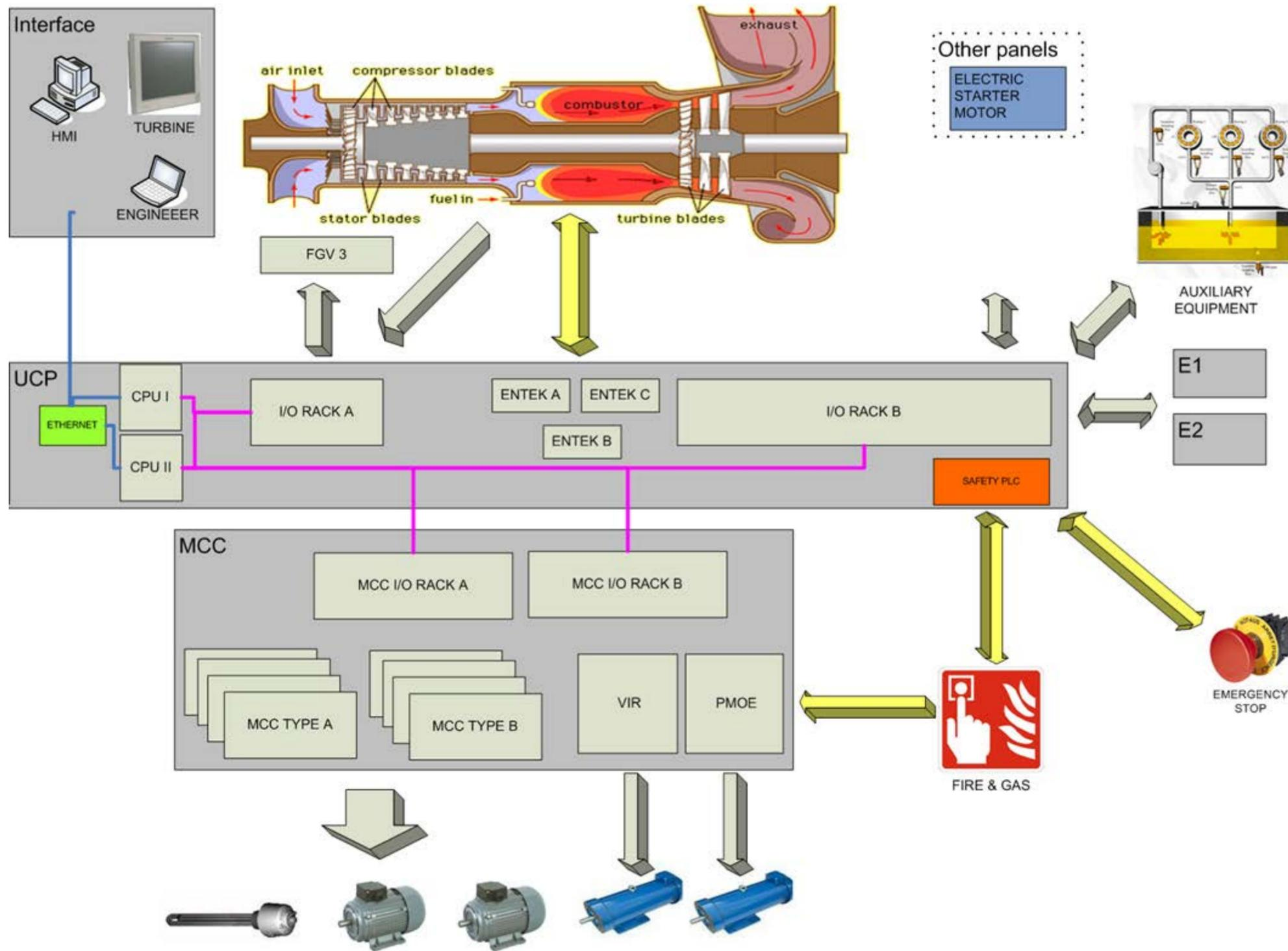
Figure 4-2 : Control System Architecture
