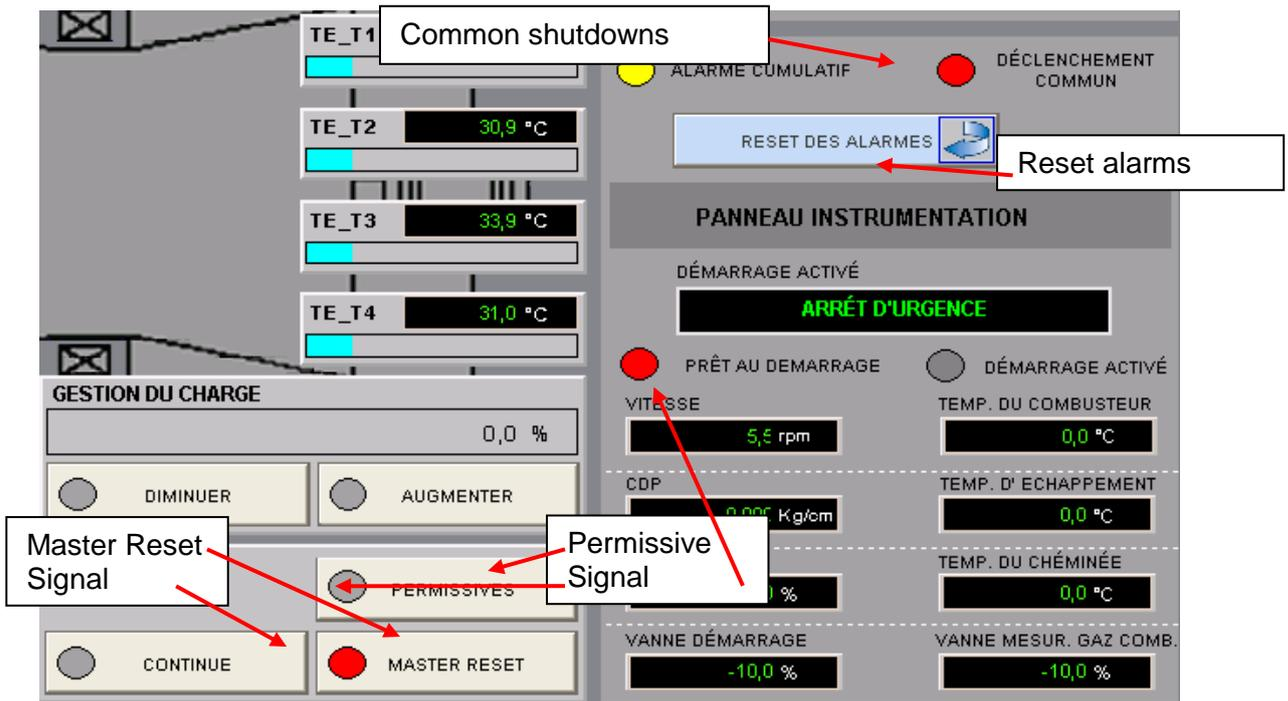
**Figure 6-6 Reset triggers**
