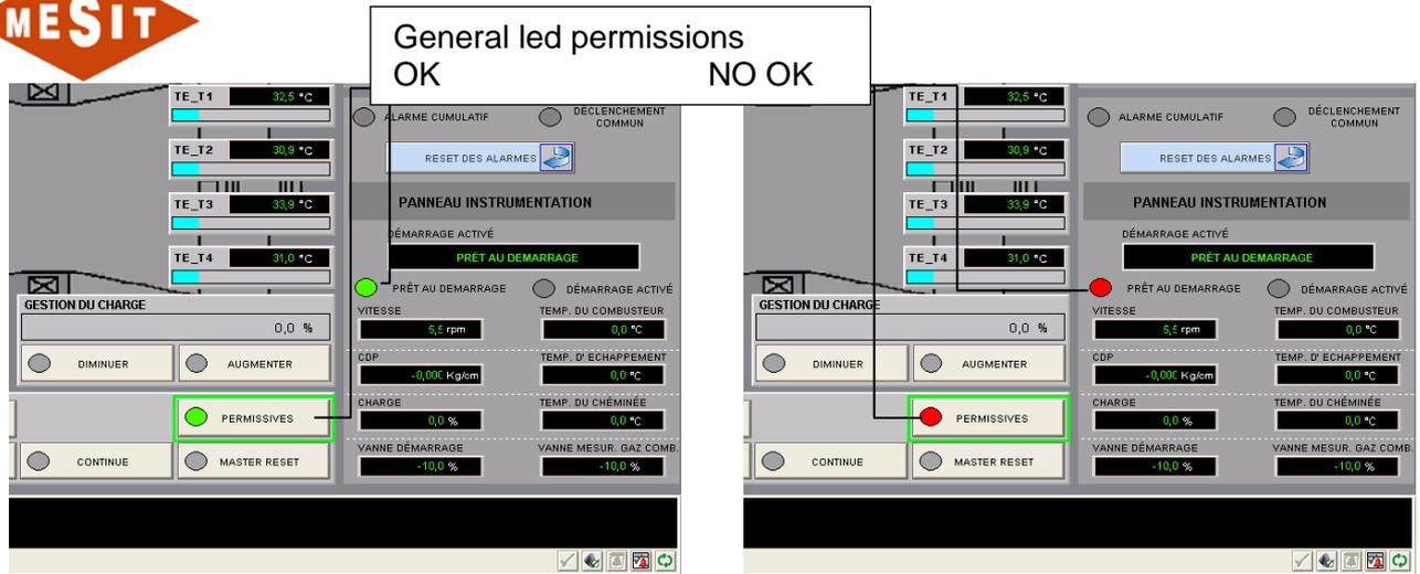
Figure 6-4 Signalling permissions
