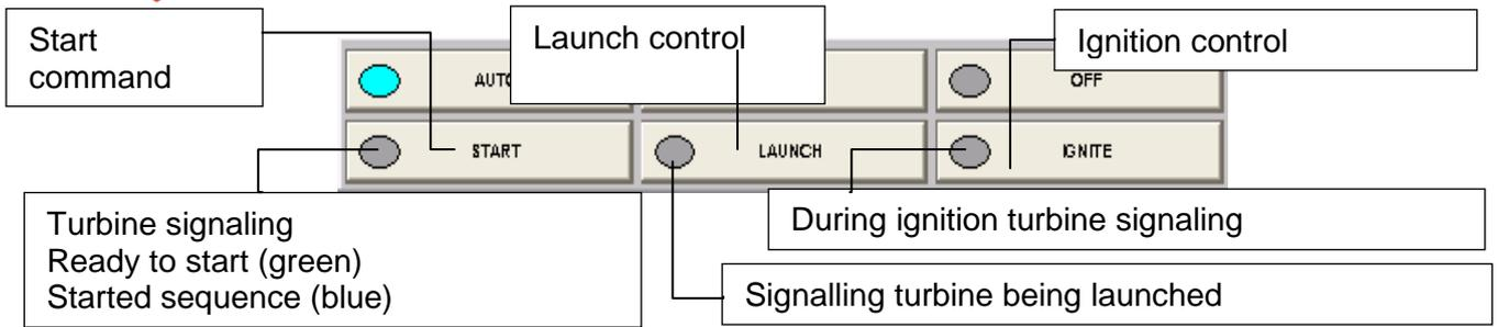
**Figure 6-6-7 Commands and signals starting phase**
